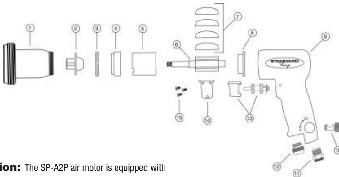
**Description:** The SP-A2P air motor is equipped with a plate which permanently locks the trigger in the "ON" position. The speed of the motor can be adjusted by turning the speed regulator on the side of the motor handle between the "OFF" position and the "MAX" position.
